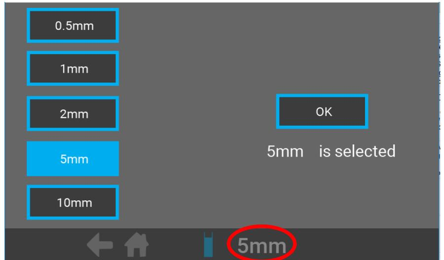
The cuvette path selected will appear at the bottom of the screen.
