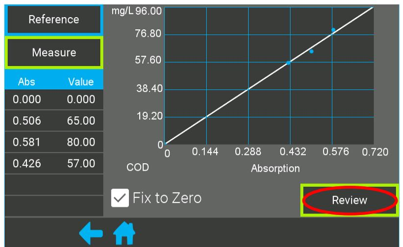
Edit the Max Value of the measurement. For example, if the three calibration points fall below what you expect the Max Range to be, then enter the Max Range of your water.
