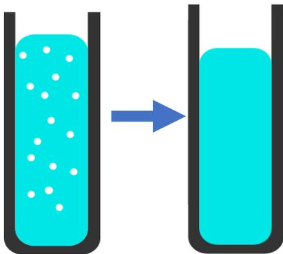
Gently tap the cuvette on a flat surface to remove any bubbles from the sample
