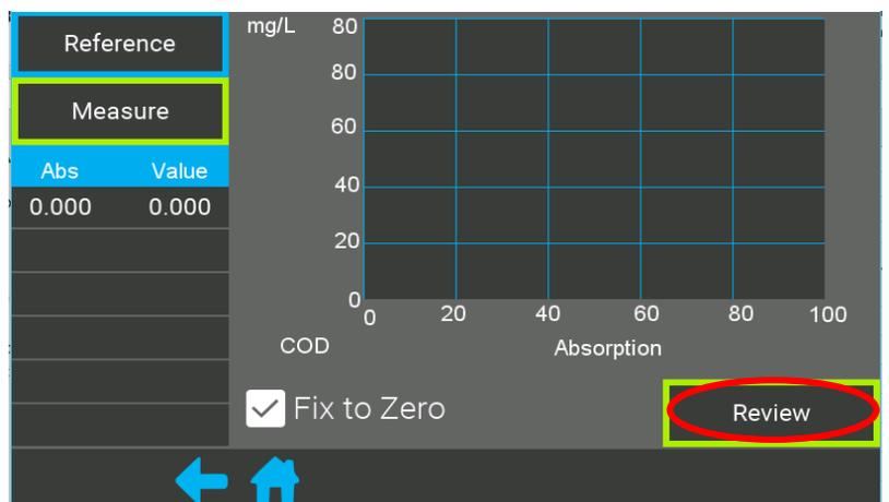
Click measure and then enter the value for sample 1. For example, if sample 1 was 65mg/L from the photometer enter it in the box show below.
